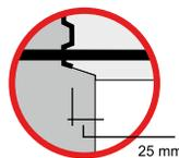
Type RSH is installed with a planned 25 mm recess
